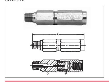
**Piston Type:** Shocks and pulsations are absorbed in the doughnut-shaped orifice (0) formed by the piston (P) in the tube. As the piston moves up and down with the pulsation, it automatically clears away any sediment or pipe scale that would clog a simple orifice or needle valve.
