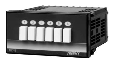
The Trerice TR\$16 Selector Switch is the ideal accompaniment for the Trerice TRD16 Digital Indicator. The TRS16 allows economical measurement of multiple individual processes (using the same thermocouple type) while requiring only one digital indicator. The push buttons indicate which process measurement is currently displayed on the indicator. Size is 96 mm x 48 mm (1/8 DIN).
