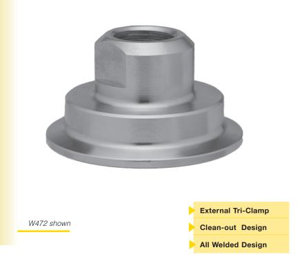
The Trerice **Sanitary Diaphragm Seal** is intended for use in the food and pharmaceutical industries, or in any application where a thorough cleaning of the wetted surface is required. Ease of maintenance is ensured as surfaces that contact the process media are virtually free of crevices. The all welded construction and external Tri-Clamp connection allow for easy removal and cleaning.
