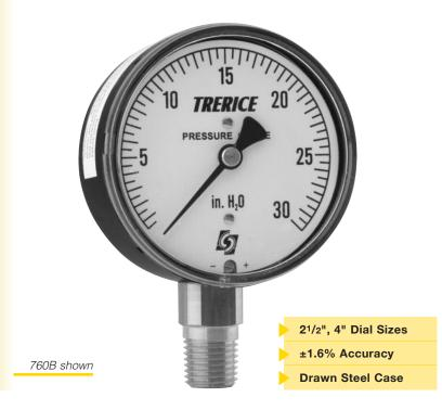
The Trerice **760B** Low Pressure Gauge is designed to accurately measure extreme low pressure conditions. This pressure gauge employs a diaphragm capsule sensing element to measure the low pressure. Case material is drawn steel with brass wetted parts.
