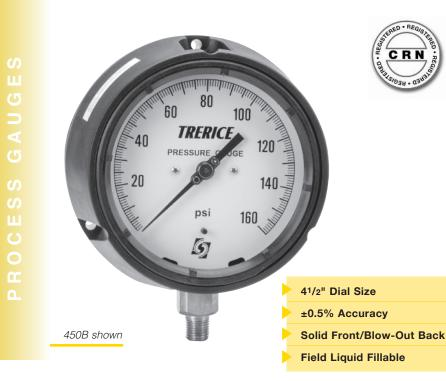
The Trerice 450 Series Process Gauge is designed for the petrochemical and industrial process industries. This solid front, blow-out back gauge is noted for its fiberglass reinforced polypropylene turret case and screwed ring; its sturdy interior design; and its field liquid-fill capability (no kit required). The 450 Series can withstand the most rugged industrial applications, while maintaining precise accuracy. Wetted parts are bronze tube/brass socket, stainless steel, or Monel.
