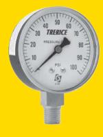
The Trerice 800B Utility Gauge is designed for general pressure indication requirements. This gauge provides excellent accuracy (1.6% full scale) and reliability at an economical cost. The case is drawn steel and wetted parts are brass.
