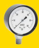
Trerice Low Pressure Gauges are essential for accurately measuring low pressures such as natural gas. This gauge employs a diaphragm capsule element to accurately measure pressures of 10 psi or below. The case is drawn steel with brass wetted parts.
