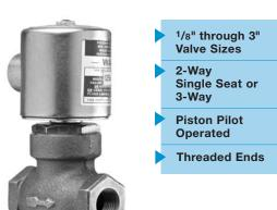
The Trerice **960 Series Solenoid Valve** is particularly suited for use with electric contact controllers. This packless, self-contained valve is designed to operate on a minimum of current and can be used for air, steam, water, oil other liquids that are not corrosive to brass. The valve is opened and closed by a balancing piston and is controlled by a small pilot valve. The Series 960 should always be mounted to a horizontal pipeline with the coil in an upright position.
