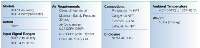
Valves with positioners operate on a control signal of 3-15 psig or 4-20mA and utilize an internal 9-15 psig range spring.
