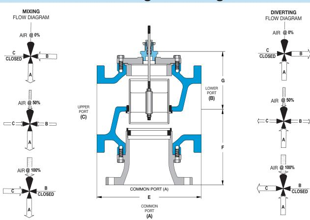
Trerice 3-Way Valves are not designed for use in steam applications. To properly control the mixing of two flows, inlet pressures at ports B and C should be as equal as possible.
