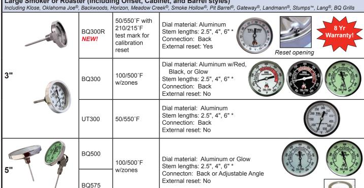
Installation: The above models have a 1/2" NPT connection which threads into a welded coupling or installs into a 7/8" diameter hole with washer and nut (sold separately p/n 4903101). \* Select a 6" stem for an insulated cooker.
