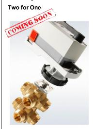
The Siemens 6-way control ball valve is suited for use in heated / chilled ceiling applications. This special design replaces four conventional valves and respective actuators in a 4-pipe heated/chilled ceiling. Since there is only actuator, it occupies only one data point. Less effort for installation, commissioning and cabling as well as decreased space requirements reduce the complexity of the plant and result in lower costs.
