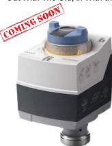
Siemens SAS Series Actuator is a direct replacement for the retired SQS series actuator. The SAS series actuator require a 24 Vac supply and can receive a 0-10 Vdc or 0-1000 Ohm control signal to proportionally control a valve, or receive a floating control signal to provide floating control. This actuator is designed to work with Powermite MT Series Valves with a 7/32" (5.5 mm) stroke. These valves can be used in liquid and low pressure steam service applications.
