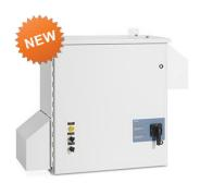
Siemens NEMA Type 3R BT300 and BT300 with bypass are recent additions to the BT300 Variable Frequency Drives (VFDs) family. Manufactured for outdoor locations, the standard 3R rating cabinet provides protection from rain to the enclosed VFD and electrical control components. NEMA 3R BT300s are available in 208-240V up to 60HP and 380-480V up to 125HP.
