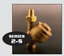
Aquatrol bellows "fail-safe" designed in the event the bellows ruptures, it expands to a closed position. The result is a "cold unit" signal for maintenance. Aquatrol's bellows is constructed of stainless steel.
