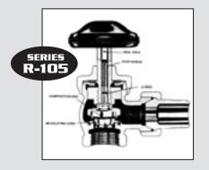
Series R-105 Valve is designed for balancing of both steam and hot water. Stop screw adjustments allow for a full range of settings without removing the valve or shutting down the system. Refer to R-100 for patterns and sizes.
