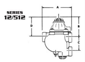
Series 12/512 and 8/508 Float and Thermostatic Traps are compact, light and esay to clean, service and install.
