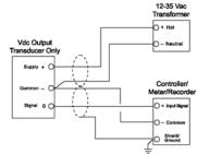
Figure 7. Wiring the VDC Output Duct Pressure Transducers
