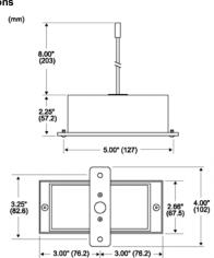
Figure 1. Duct Pressure Transducer Dimensions
