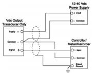
Figure 8. Wiring the VDC Output Duct Pressure Transducers With a DC Power Supply
