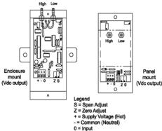
Figure 5. Pressure Transducer With VDC Output
