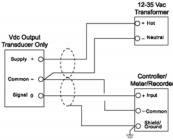
Figure 8. Wiring VDC Output Transducers With an External AC Power Supply
