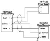
Figure 9. Wiring VDC Output Transducers With an External DC Power Supply
