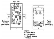
Figure 4. Pressure Transducer With mA Output
