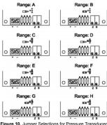
Figure 10. Jumper Selections for Pressure Transducers With mA Output
