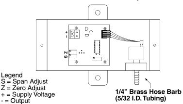
Wiring PR-243 Units with VDC Output
