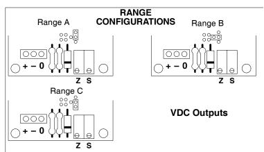
Figure-6 Jumper Selections for Pressure Transducers with VDC Outputs.
