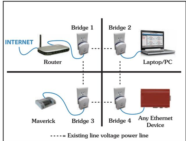
*Just plug it in and connect - No new wires*
