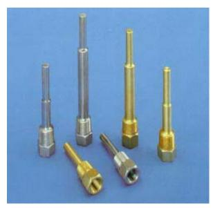
The A-500 Thermowell is machined from a single piece of brass or stainless steel to provide a rugged and leak proof well for MAMAC temperature sensors. Each A-500 Thermowell is precisely machined to 0.255" bore to provide a tight fit for our standard 1/4" O.D. probe. This feature also significantly enhances the thermal transfer from the media to the temperature sensor.
