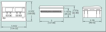
Simultaneously measure and control temperature and humidity with the Series THC Temperature/Humidity Switch. The unit offers a 3-digit red display for temperature indication and a 3-digit green display indicating humidity. The Series THC is equipped with four independent relays, two for temperature control and two relays for humidity control.
