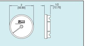
**Measure the temperature** of boilers, air ducts, motors, bearings, furnaces or other surfaces with Series ST Surface Mount Thermometers. Dual magnet design allows easy mounting on any ferrous surface. Bi-metallic thermal sensing coil provides quick temperature measurement with  $\pm 2\%$  full scale accuracy.
