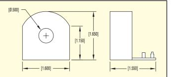
**Love Controls Series LTTJ Current Transformers** allow easy monitoring of the current flowing to your load. This easy to use device provides a 0 to 10 VDC signal into both low and high impedance circuits, and is easily scalable to your needs.
