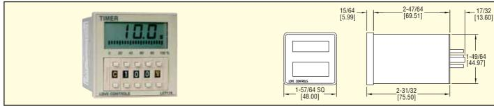
**The LCT116 Digital Timers** provide simple, yet economical solutions for a variety of timing applications. Installation is simple with compact 1/16 DIN package. Set point and timing functions are easily adjusted with the individual set buttons. A LCD display on the front indicates current time status and a bargraph for indicating relative time remaining. Ten different timing functions and ten different time scales give you the greatest flexibility.
