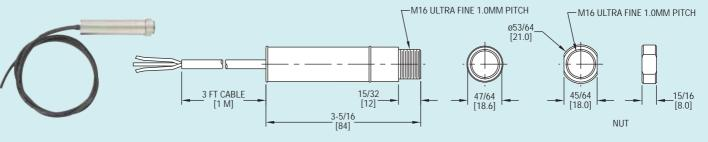
**The Series ILA Non-Contact Sensors**, measure temperatures from 32 to 932°F (0 to 500°C) and provide a linear 4 to 20 mA, 0 to 50 mV VDC or thermocouple output. The 2-wire signal is compatible with almost any indicator, controller, recorder, data logger, etc., without the need for special interfacing or signal conditioning. They are suitable for most materials such as food, paper, textiles, plastics, leather, tobacco, pharmaceuticals, chemicals, rubber, coal, and asphalt.
