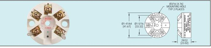
Series 659 Push-Button Temperature Transmitters accept thermocouple (J. K. T). RTD  $(Pt100\Omega)$  or thermistor input and provide a linearized 4 to 20 mA output. The transmitter is quickly ranged and calibrated by using a single on-board switch. An LED provides visual indication of sensor fault and programming mode. Models feature reverse polarity protection. Thermocouple models are also galvanically isolated and cold iunction compensated.
