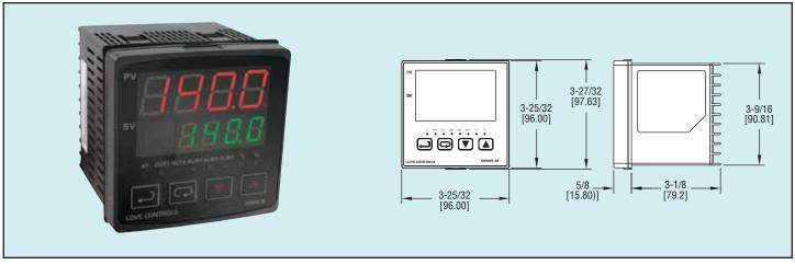
The Series 4B 1/4 DIN Temperature/Process Controller is designed to accept thermocouple, RTD, current or voltage input and provide dual outputs for control. Available outputs include relay/relay, voltage pulse/relay, current/relay, or linear voltage/relay.
