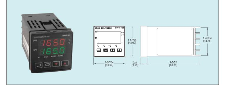
The compact Series 16C Temperature Controller offers accurate temperature measurement and control in a 1/16 DIN package. Designed for direct or reverse acting (cooling or heating) control, the Series 16C can be programmed for simple ON/OFF or more complex PID control functions. PID control is supported with manual or auto-tuning. Select relay, voltage or current output for control methods.
