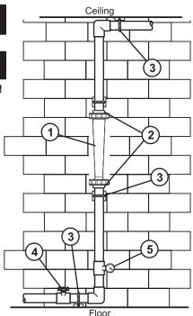
tools. Union nuts should be hand tightened only. DO NOT OVER-TIGHTEN!
