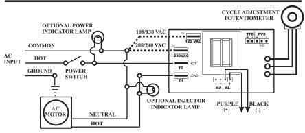
WIRING DIAGRAM - Model A-100NA & A-100NC
