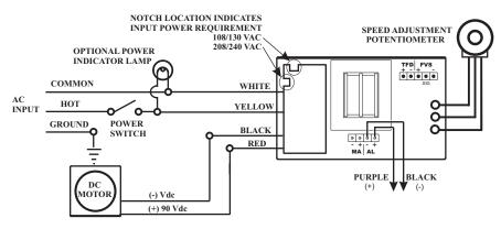
WIRING DIAGRAM - Model A-100NF
