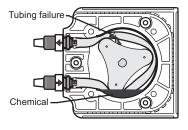
the pump head - just enough to cover the sensors. Turn on the pump. If the TFD system detects the chemical, the pump will stop after a five second confirmation period. If the TFD system does not detect the chemical, the pump will continue to run after the confirmation period. Carefully clean the chemical out of the pump head being sure to remove all traces of chemical from the sensor probes. Turn the power switch off and on to reset the pump.
