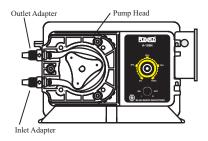
**Install the New Pump Tube** - Be sure the pump head chamber is clean and free of any debris.
