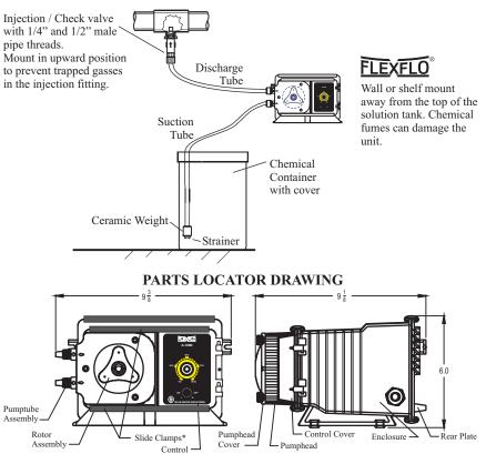
\* Slide both top & bottom clamps to the left only far enough to open the control cover.
