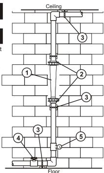
**3.** Wall, floor and ceiling mounts and supports are to be carefully aligned and sturdy. Wall, floor and ceiling supports are recommended as needed. This is to maintain pipe alignment and to prevent vibration.
