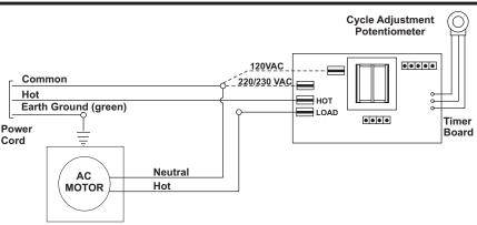
FIG. 4.6 WIRING DIAGRAM - FIXED TIMERS
