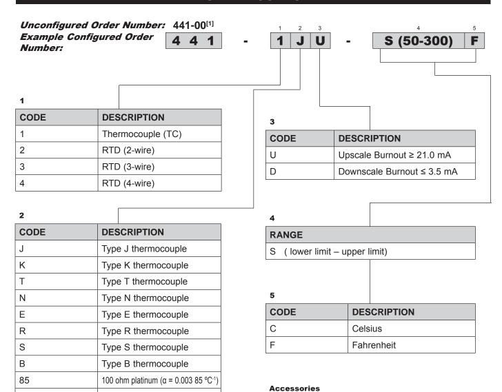
[1] Default setting for unconfigured transmitter is 3-wire Pt100 (0 - 100) °C.
