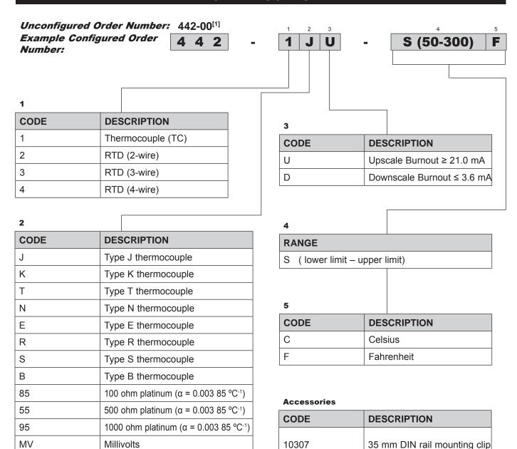
[1] Default setting for unconfigured transmitters is 3-wire Pt100 (0 - 100) °C.
