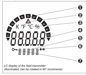
Item 1: Bar graph display in 10% increments with indicators for overranging / underranging
