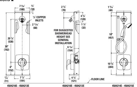
The recommended minimum distance between the centerline of two HydroPanel<sup>®</sup> II units is 36" (914 mm). Position units evenly between inlet supply piping. Suggested showerhead heights (if not shown on architectural plans for shower room) are:
