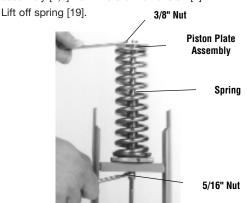
9A. (1/2" TO 2") REMOVE PISTON PLATE AND SPRING
