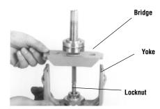
10B. (2-1/2" TO 4") LIFT OFF BRIDGE AND YOKE
