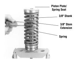
9B. (2-1/2" TO 4") REMOVE PISTON PLATE/SHANK AND SPRING
