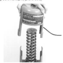
8. REMOVE HOUSING AND THERMAL SYSTEM
