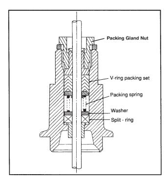
Figure 1. V-Ring and Split Ring Packing
