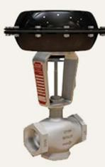
Modern manufacturing techniques and modular construction allows these stainless steel valves to be extremely cost-effective in comparison to valves with bronze, cast iron or cast steel bodies. The standard configuration has an equal percentage flow characteristic with metal-to-metal seating, spring-loaded Teflon V-ring stem packing and pneumatic actuator. The HB Series is available with both pneumatic or electric actuation.
