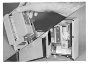
**6.** Replace the #4-128 Firetron cell in the scanner with the #4-263 firetron cell. Attach the label supplied with the 4-263 Firetron cell to the scanner body.
