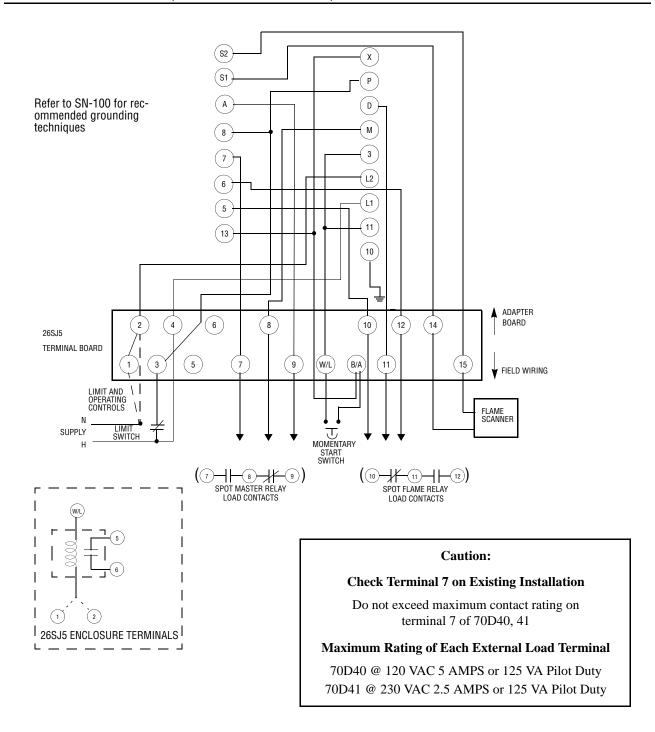
**Note:** Fireye 26SJ5 Controls include a SP-N.O. load circuit at terminals 5 and 6, which cannot be included when a PD4 Modernization Adapter Kit is used. If the 5-6 circuit function is desired, add auxiliary relay, connection as shown above. The terminal board pins on the 60-2060-4 Adapter at terminals 5 and 6 have been removed.
