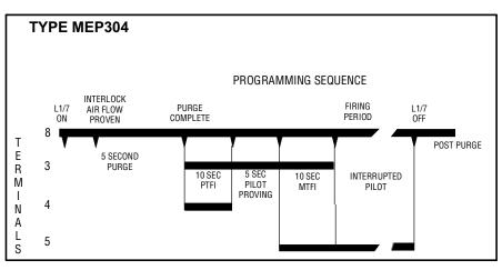
0 Second post purge on operating control open. 15 Second post purge on flame fail. Non-recycle operation on flame fail.
