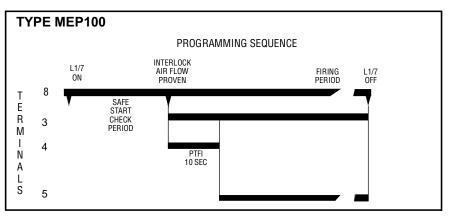
Terminal #5 is energized 3 seconds after flame is detected. Re-ignited PTFI on flame fail after Terminal 5 energized. Recycle on loss of interlock (air flow) after flame proven.
