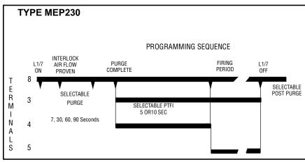
Terminal #5 is energized 3 seconds after flame is detected. Selectable Recycle/Non-Recycle operation on loss of flame after Terminal 5 energized. Recycle on loss of interlock (air flow) after flame proven. Selectable air flow (interlock circuit) proven at start.
