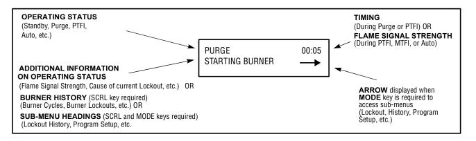
At any time the MicroM is powered, the SCRL key is used to scroll through and display the total number burner hours, burner cycles, burner lockouts and system hours on the bottom line of the ED510 display. The top line will continue to show the current run mode of the control (e.g. PURGE, AUTO, etc.) Following the historical information, the SCRL key will display three (3) sub-menus providing the following information and/or functions:
