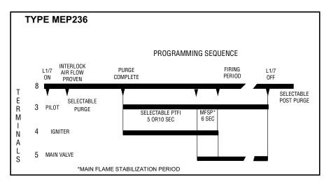
Terminal #5 is energized 3 seconds after the flame is detected.
