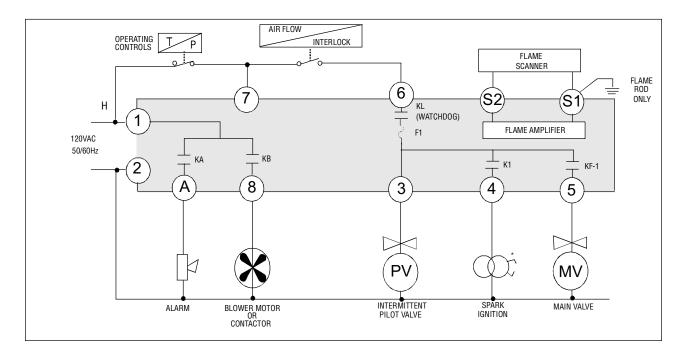
FIGURE 8. WIRING ARANGEMENT FOR DIRECT SPARK IGNITED BURNERS, TWO STAGE OPERATION USING MEP100 AND MEP200 SERIES PROGRAMMERS
