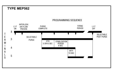
Pilot stabilization timing begins as soon as flame is proven.
