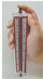
For high scale reading, finger covers hole
