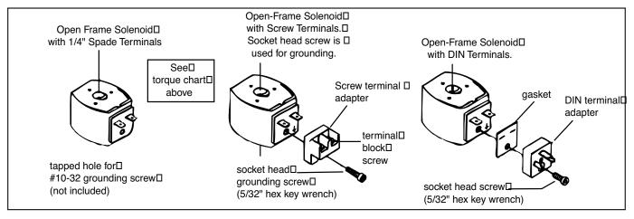
Figure 4. Open - frame solenoids
