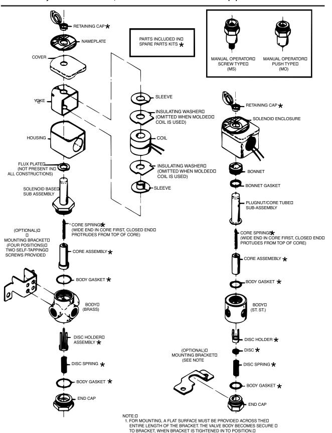
IF THE VALVE HAS A MANUAL OPERATOR, A HOLE MUST BE MADED THROUGH THE MOUNTING SURFACE FOR THE OPERATOR STEM.
