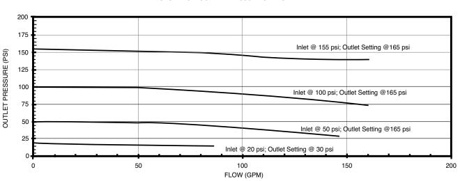
1-1/2" 90G-21 OBSERVED FLOW RATE WHEN INLET PRESSURE DROPS BELOW OUTLET PRESSURE SET POINT
