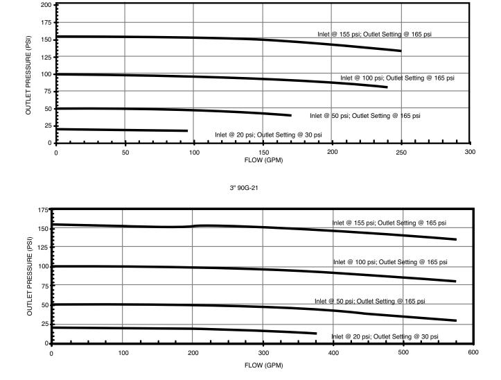
2" 90G-21 OBSERVED FLOW RATE WHEN INLET PRESSURE DROPS BELOW OUTLET PRESSURE SET POINT
