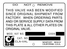
This aluminum plate is included in pilot system modification kits and is to be wired to the new pilot control system after installation.
