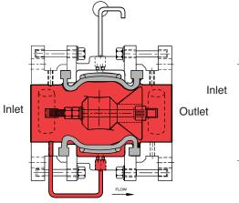
**Full Open Operation** The valve opens when pilot set pressure is reached and pressure in the control chamber is relieved.
