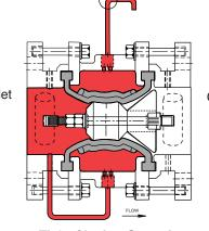
**Tight Closing Operation** Water pressure (equal to inlet pressure) from valve inlet or from upstream of valve is applied to the control chamber. Valve closes bubble tight.
