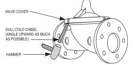
On 6" and smaller valves block and tackle or a power hoist can be used to lift valve cover by inserting proper size eye bolt in place of the center cover plug. on 8" and larger valves there are 4 holes (5/8" - 11 size) where jacking screws and/or eye bolts may be inserted for lifting purposes. **Pull cover straight up** to keep from damaging the integral seat bearing and stem.
