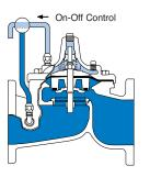
**Full Open Operation** When pressure in the cover chamber is relieved to a zone of lower pressure, the line pressure at the valve inlet opens the valve, allowing full flow.
