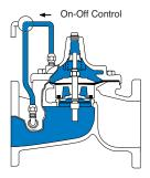
**Tight Closing Operation** When pressure from the valve inlet is applied to the cover chamber, the valve closes drip-tight.
