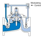
Modulating Action The valve holds any intermediate position when operating pressure is equal above and below the diaphragm. Using a Cla-Val "Modulating" Control will allow the valve to automatically compensate for line
