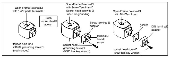
Figure 4. Open - frame solenoids
