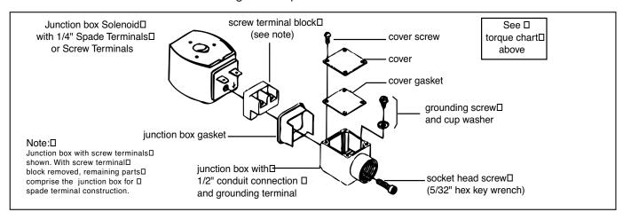
Figure 5. Open - frame solenoids
