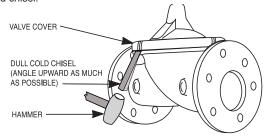
On 6" and smaller valves block and tackle or a power hoist can be used to lift valve cover by inserting proper size eye bolt in place of the center cover plug. on 8" and larger valves there are 4 holes (5/8" — 11 size) where jacking screws and/or eye bolts may be inserted for lifting purposes. **Pull cover straight up** to keep from damaging the integral seat bearing and stem.
