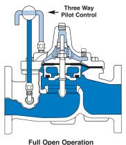
When pressure in diaphragm chamber is relieved to a zone of lower pressure (usually atmosphere) the line pressure (5 psi Min.) at the valve inlet opens the valve.
