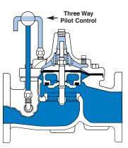
**Full Open Operation** When pressure in diaphragm chamber is relieved to a zone of lower pressure (usually atmosphere) the line pressure (5 psi Min.) at the valve inlet opens the valve.
