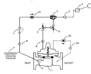
The "D" feature on a vertically installed 6" and larger valve must be horizontally installed.
